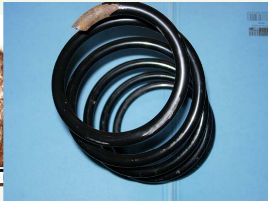
Fracture of a motor car spring as a consequence of fatigue corrosion due to cyclic loadings and a corrosion caused by a media in winter time conditions.
