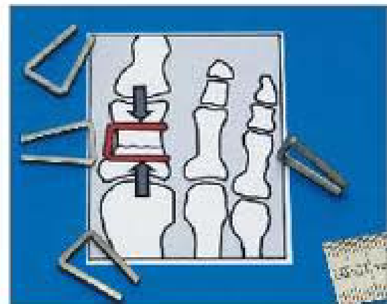
Foot staple used for clamping bone fractures produced from NiTi shape memory alloy (Courtesy Forschungszentrum Jülich, Germany)
